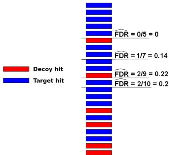
Figure 3. Illustration of how FDRs can be estimated using a composite target-decoy DB (from the work describing the method MUMAL by Cerqueira et al. (52)). In this example, only one score (univariate analysis) is used. The hits are presented in descending order, i.e. the highest score is on top. For a given threshold value, the number of decoy hits with score greater or equal to this value is used to estimate the number of wrong matches among target hits obtained using the same threshold.
