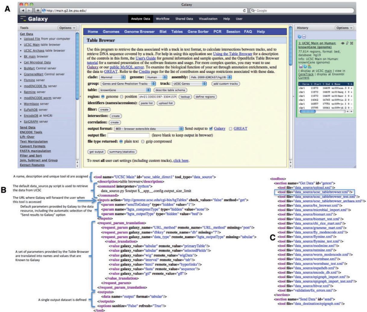
Figure 1. The UCSC Table Browser tool. The UCSC Table Browser tool is shown with its native interface as it appears integrated into Galaxy (A). A simplified XML configuration file (B) that describes to Galaxy how to communicate with the data resource is shown. Advanced configuration options have been used to customize data set attributes and to enhance the user experience. Values for the file format and genome build are taken from the parameters provided by the datasource and made accessible to Galaxy. Additionally, this configuration causes the 'Send output to Galaxy' option to be automatically selected when a user begins from within Galaxy. The addition of a single line, outlined in blue, to the tool_conf.xml file is all that is required to inform Galaxy to load the tool (C).
