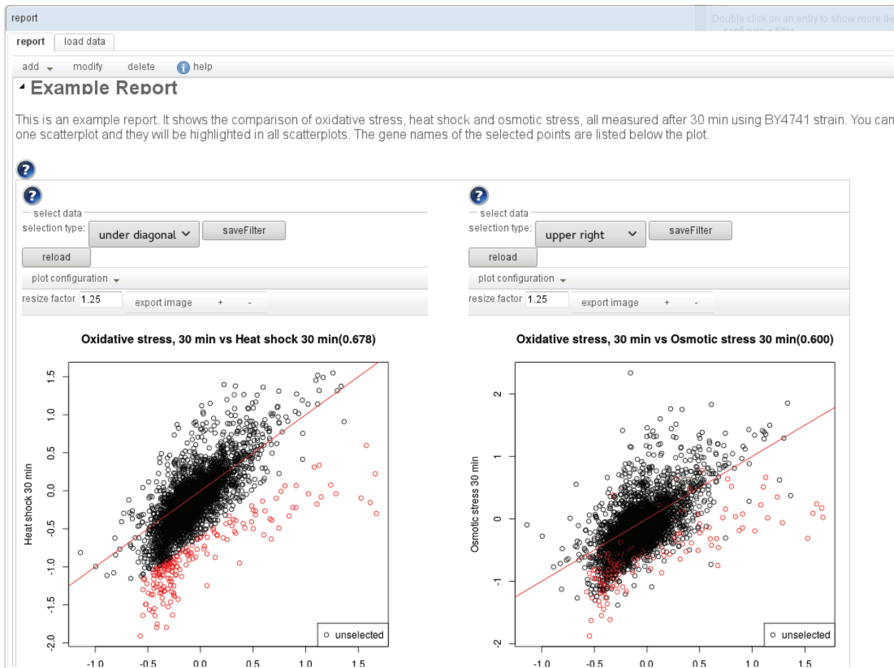
Figure 3. An example report: A report consists of sections, with text and interactive visualizations. An editor allows one to modify/add/delete the individual elements and to change their order. Many of the available visualizations are also interactive. E.g. in the scatterplot shown here, sets of genes can be selected to highlight them (also in other subplots of the visualization) and to display the labels of the selected points in a list below the plot.
